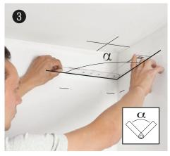
**Determine the angle** I Read the size of the angle using our protractor FB15.
